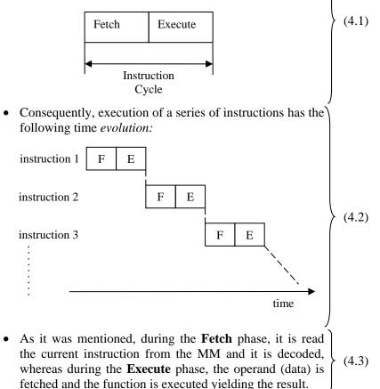
• The prefetching procedure consists in *overlapping* the **Execute** phase of the current instruction with the **Fetch** phase of the next instruction, provided that there are no requests of common resources.
