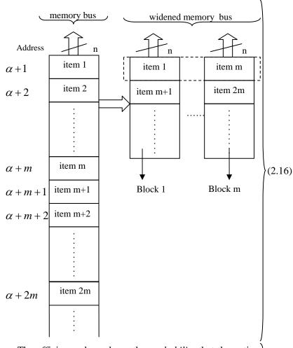
• The efficiency depends on the *probability* that the entire set of instructions in a widened word  $(n \cdot m)$  to be used by the CPU; frequently, there are *branches in the program evolution* that require a change of the normal sequence of instructions. Then a new access to the block of memories will be initiated to fulfil requirements of the branch, before all instructions / data from the previous word had been executed by the CPU.
