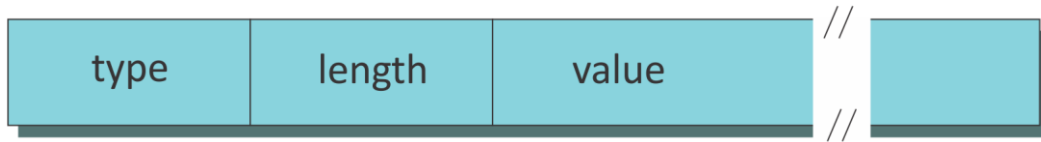
Fig. 2.19. IPv6 Type-Length-Value (TLV) option format
